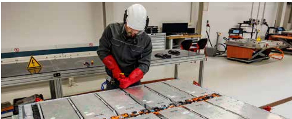
A Volkswagen engineer disassembles used EV batteries for material recovery.
