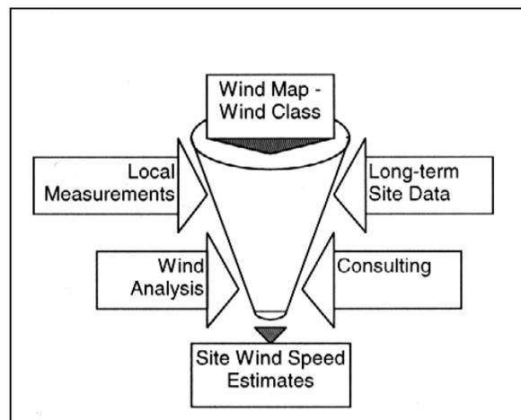
**Figure 1.** You might think of the wind assessment process as a funnel where rough estimates of wind power class from wind maps go in one end and more refined and precise estimates of site-specific wind speed come out the other end.
