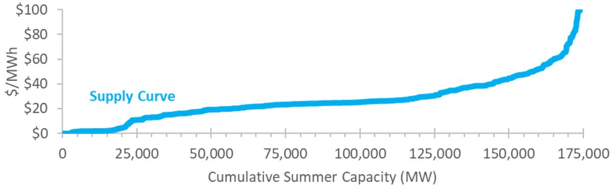
MISO's 2019 supply curve shows all available resources in the system being lined up from lowest cost to highest cost (merit order).
