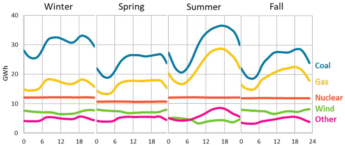
While coal generation is present all day and all year, at least some of the coal is forced to cycle up and down to follow load patterns. Operationally, significant portions of coal capacity in MISO no longer operate as traditional baseload resources. SOURCE: UCS, BASED ON DATA FROM S&P GLOBAL 2020.
