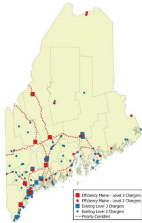
Public EV Charging Infrastructure (Source: Efficiency Maine )
