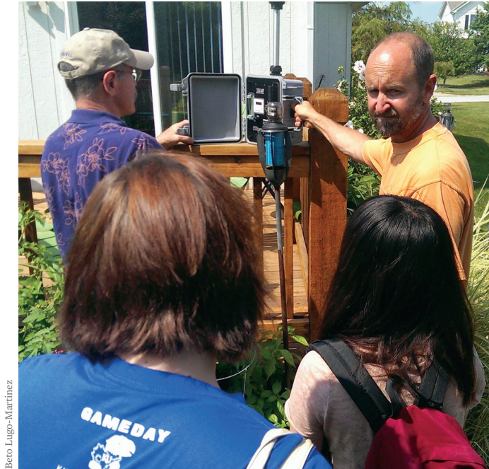
CleanAirNow installed air monitors in Kansas City communities to measure pollution levels in residential areas. The results show that pollution levels are often higher than indicated by federal air monitors that don't capture spikes in air pollution near freight corridors and industrial facilities.
