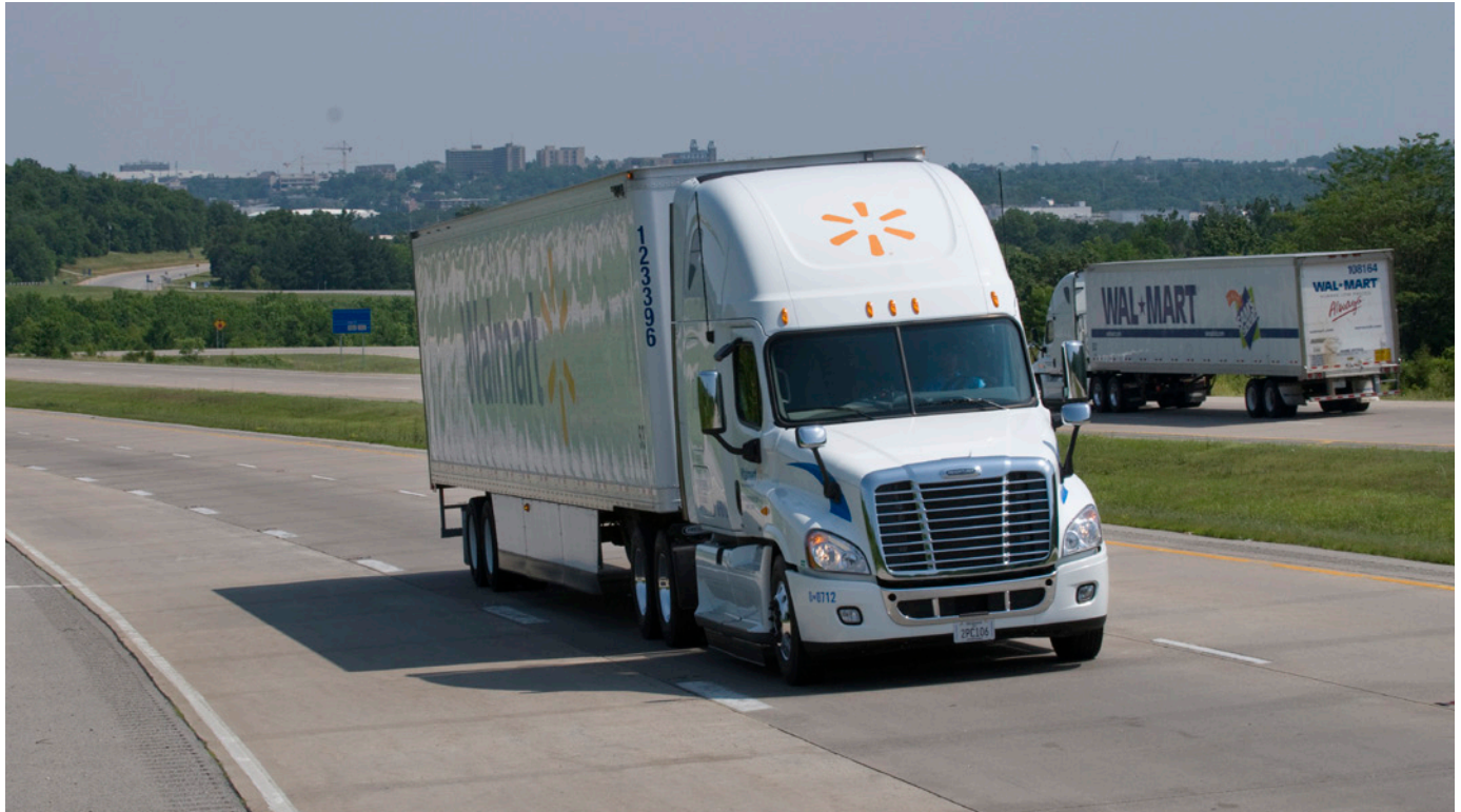
Walmart's tractor-trailers are a critical component of its just-in-time delivery model. The skirts on the tractor and trailer as well as more aerodynamic design of the tractor help reduce fuel use from these large trucks.
