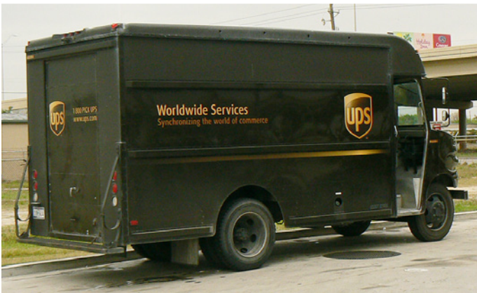
Heavy-duty trucks of all shapes and sizes move freight around the United States. Tractor-trailers (top left) include both line-haul trucks, which travel hundreds of miles daily, and regional-haul trucks, which typically operate within 200 miles of a central location. Other heavy-duty vehicles include box trucks (top right); step vans, commonly known as delivery vans (bottom left); and cargo vans (bottom right).
