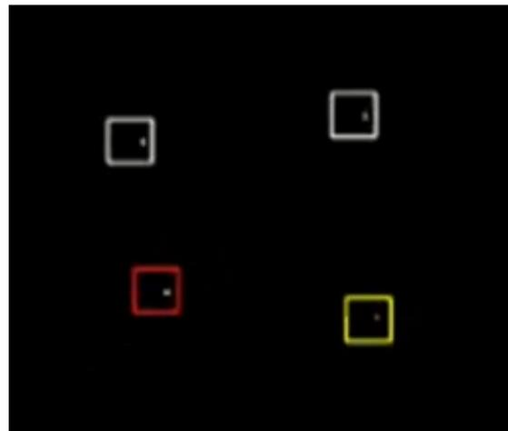
*A still from a video showing the objects in the target cluster of FTG-06B as seen by the kill vehicle's sensor (1:26 into video). The decoys are in the light blue squares, the missile stage is in the yellow square, and the mock warhead is in the red square*
