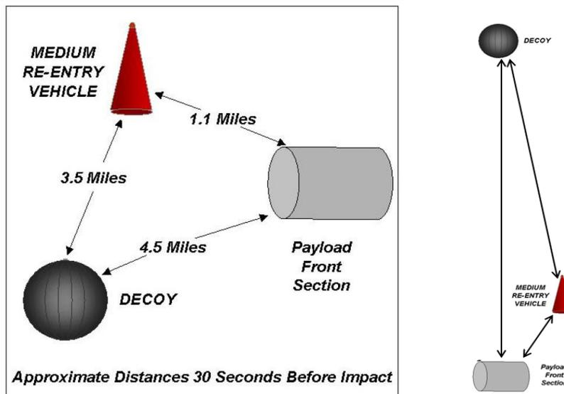
The diagram on the left is from the Pentagon briefing on IFT-6 (the “payload front section” is the upper booster stage that released the warhead and balloon). SOURCE: Nance 2001. The diagram on the right shows the actual separation of the objects in the plane that contains them.
