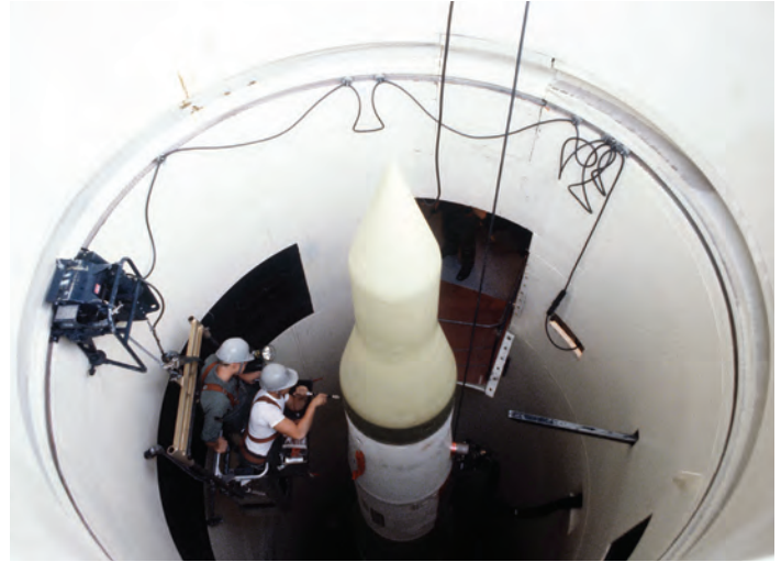
Two U.S. Air Force missile maintenance crewmen perform an electrical check on a Minuteman III intercontinental ballistic missile in its silo at Whiteman Air Force Base in Missouri.
