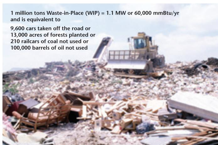
1 million tons Waste-in-Place (WIP) = 1.1 MW or 60,000 mmBtu/yr and is equivalent to
